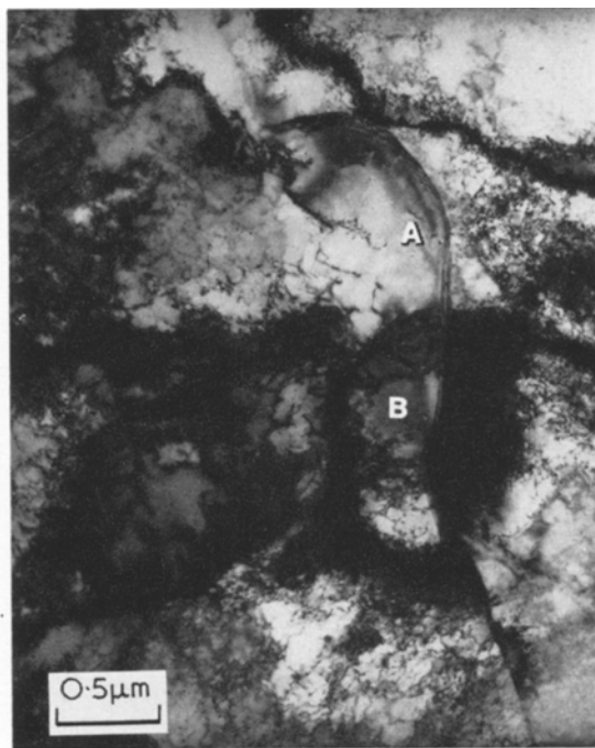
Figure 8 Cu-0.04 at. % Ag-1.2 at. % Al annealed for 60 sec at 450°C after 50% rolling.
