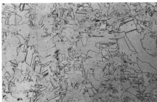
Figure 12 Completely recrystallized structure in Cu-0.04 at.% Ag-0.1 at.% Al alloy ( \times 80 ).
